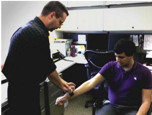
Figure 3 Example of muscle force clinical test. The subject is asked to produce maximal elevation force, and the clinical assistant restricts the motion of the subject with a MicroFet2 wireless digital handheld dynamometer. The force generated is then recorded.
